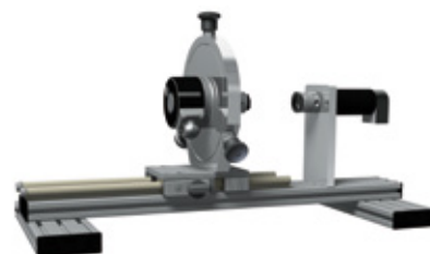
Test bench with drive motor and encoder. The Encoder is installed on an exchange adaptor.
