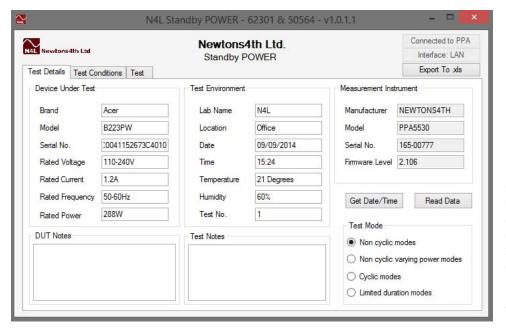
N4L Standby Power Software presents the user with an ir interface. The Brand, Model, Serial number, Rated Voltaç Frequency and Power are all inputted.
