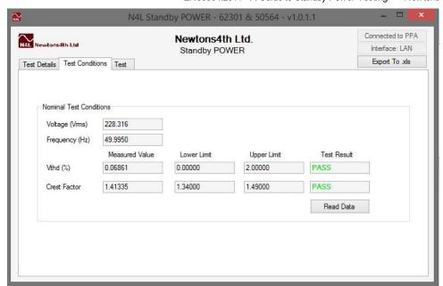
At this stage we recommend that the device under test b connected to the output of the AC source and set to stan This will result in the initial tests of the AC source being a under test conditions and will be representative of the bel AC source during the test. There is little benefit in testing source with zero load as the test results may not be represented on-load output waveform of the Power Source.
