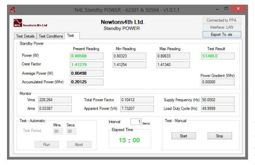
The user interface of N4L Standby Power software offers information useful to the test engineer. The accumulated continuously analysed and the power gradient (analyzed & EN50564:2011) is continually updated. In this test the powar very low after 15 minutes and a result of 0.00000 (ze decimal places) was displayed.
