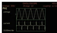
While a precise measurement in power applications generally requires the use of a numeric presentation, the SCOPE mode provided by the PPA1500 is a valuable aid to development and test.
