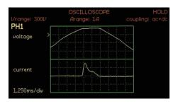
Display of voltage and current on a single phase or all three phase waveforms can be selected with user control of trigger level, pre trigger, timebase and cursors.
