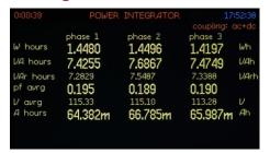
When the INTEG mode is selected, true and fundamental values of all integrated values are presented. Using the NEXT and BACK buttons, any individual phase or the sum value of all phases can be viewed.
