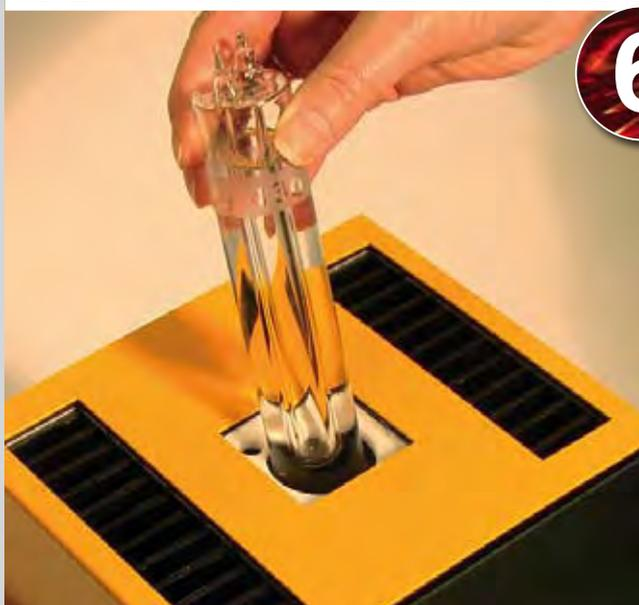
For the best possible performance with uncertainties to 0.0005°C (0.5mK) add an ITS-90 Fixed Point Cell. The most popular is the B8 Water Triple Point Cell, it is surprisingly affordable and simple to use - the triple point can be both created and maintained in the apparatus without the need for any other equipment or supplies.
