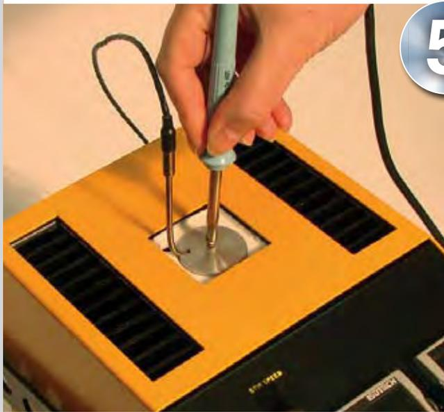
With the Surface Sensor Kit the test sensor is compared to a platinum resistance thermometer located just below the surface of the block. Again save the cost of buying additional equipment by adding accessories as required to expand the ISOCAL-6 for new calibration applications.
