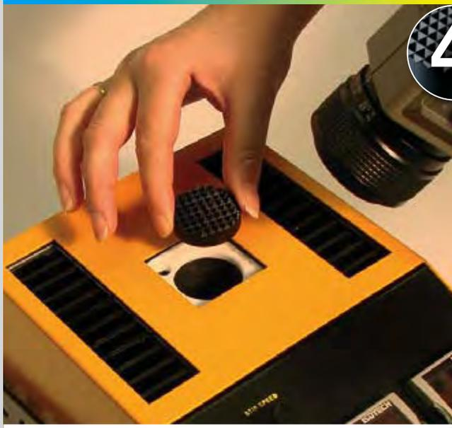
Adding the blackbody target allows the testing of infrared thermometers. Low cost non-contact IR thermometers are increasingly being used in industry and the ISOCAL-6 is ideal to test and check these devices. The IR thermometer is focused on the target and compared to a reference probe in the block pocket.
