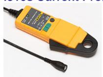
The i310s current probe is based on Hall Effect technology for use in measurement of both DC and AC current. The i310s may be used in conjunction with oscilloscopes and other suitable recording instruments for accurate non-intrusive current measurement
