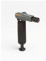
The Fluke 700LTP-1 is a hand operated pressure pump designed to generate either vacuum to -13 psi / -.90 bar or pressures to 100 psi / 6.9 bar. The Fluke 700LTP-1 has two pressure ports with quick fit connectors. Test hoses are terminated with 1/4-NPT female fittings that can be adapted using the BSP/ISO adapters.
