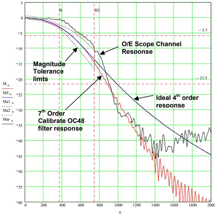
Figure 20. Transforming the O/E oscilloscope channel into the nominal 4<sup>th</sup> order Bessel Thompson response magnitude limits.
