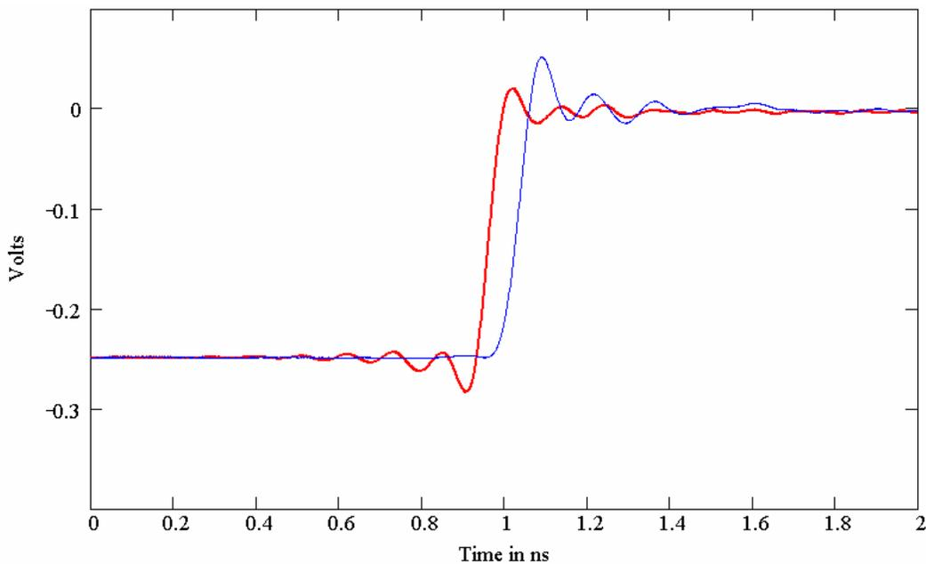
Figure 5. Comparison of step response with  $B_{W+}$  OFF in blue and  $B_{W+}$  ON in red. For this example the risetime using ET acquisition mode is approximately 46.8 ps measured using 10% to 90% levels on a 15.5 ps step generator.
