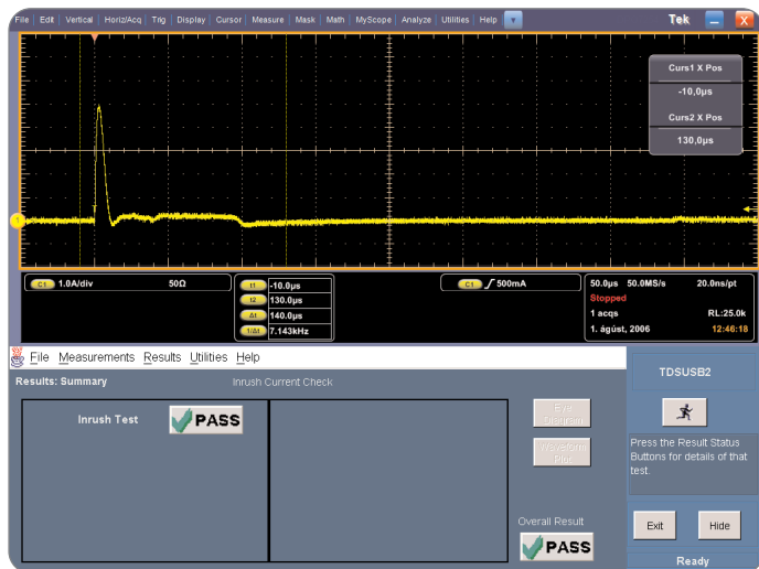
► Figure 4. Illustration of a sharp intake of current using a DP07254.
