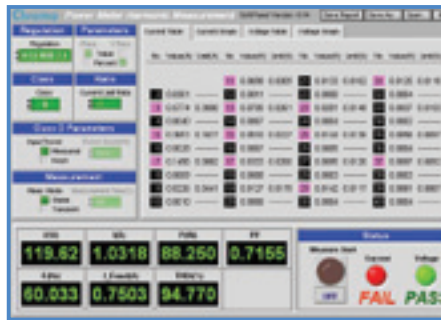
IEC 61000-3-2 Current Harmonic Test
